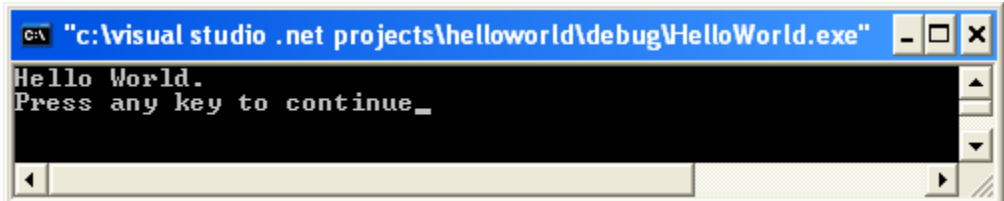
Figure 14 – Output from the execution of the HelloWorld.cpp program
